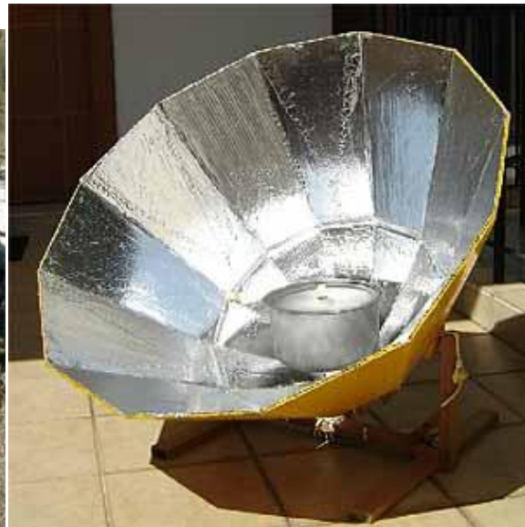
Figure 4: Different solar cooker designs have different f-ratios (the ratio of focal length to diameter).
